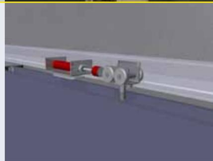
For extra safety the Palace XXL sliding wall can be fitted with the ABS. With this ABS the wall is "slowed down", providing an extra safety guarantee. The patented Parthos handle has been developed to enable the sliding walls to be opened and closed with one simple movement. It can be operated manually or fully automatically by means of a belt drive system. This variant also features automatic operation of the acoustic pressure sleeves.
